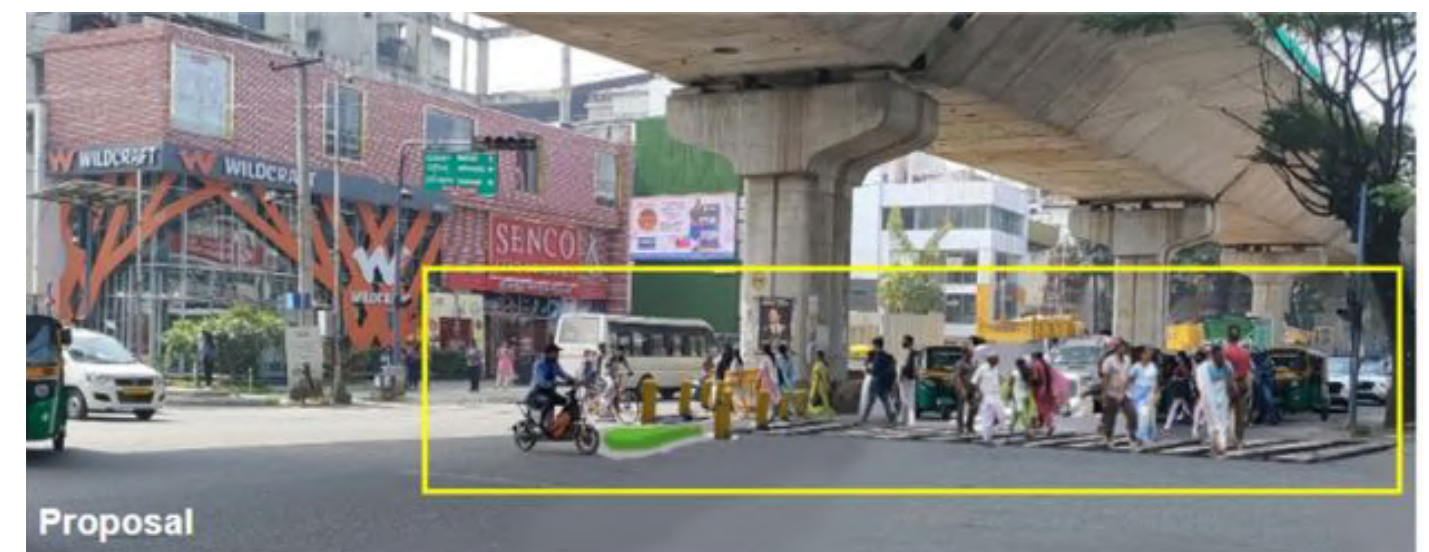
Proposed interventions for Safe pedestrian crossing at Sony World junction. Zebra crossing with median refuge island and bollards. Adequate pedestrian signal timing.
