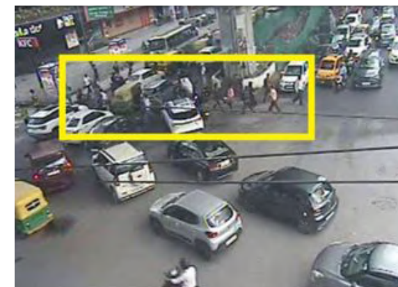
Image above: Unsafe crossing: Missing pedestrian crossing and median refuge island. Source: BTP CCTV.
