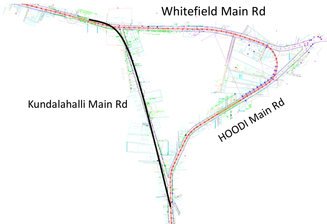
Figure 2 Metro Alignment on the Hoodi Main Road as procured form BMRCL
